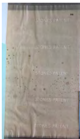
Fig. 13. Transmitted light photograph of Stones' Patent security paper, sample 102. From Illustrations of the British Paper Manufacture , Queen's University, W.D. Jordan Rare Books and Special Collections, Rare Books Collection, FF TS1105.S2.
