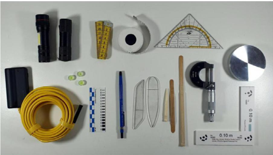
**Fig. 2.** Inspection kit for binding descriptions
